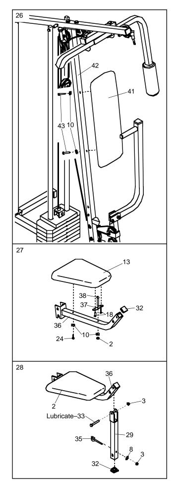
Rest the Seat Frame (36) on the indicated pin in the Front Upright (42). Attach the Seat Frame to the Front Upright with a 5/16" x 2 3/4" Carriage Bolt (14) and the Seat Knob (40).
